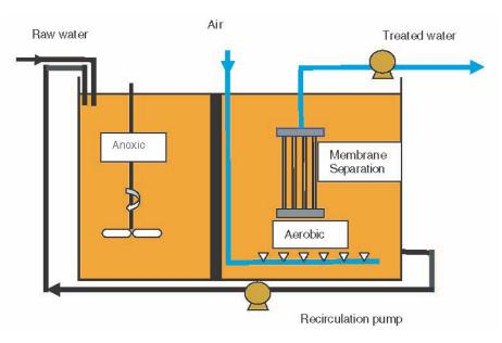
A typical MBR biological treatment system is made up of three parts, (a) an anoxic tank (where there is no or a very low concentration of oxygen), (b) an aerobic tank (where oxygen is present) and (c) a membrane separation. Wastewater is pumped into the anoxic tank and is re-circulated between the anoxic and aerobic tanks. Different types of microbes grow under the anoxic and aerobic conditions which are responsible for breaking down various contaminants present in the wastewater.
